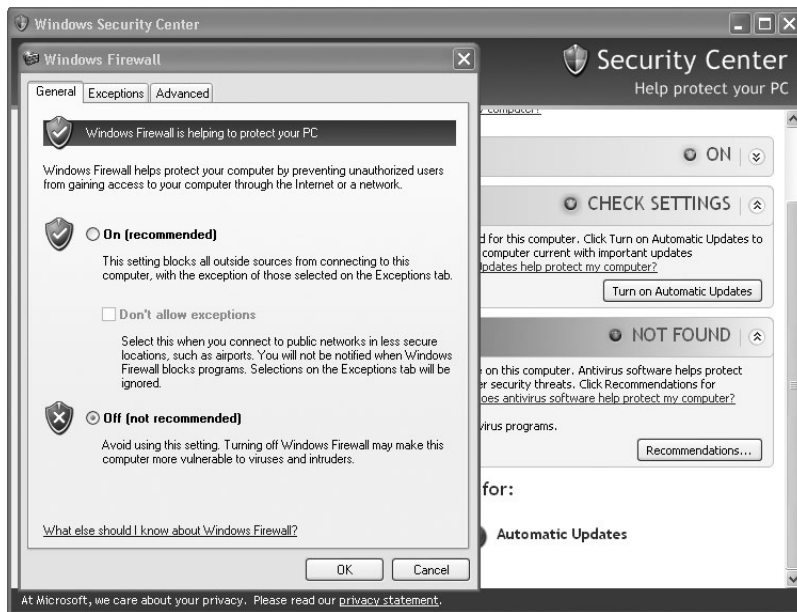
Figure 1-33: Turning off the Windows firewall
